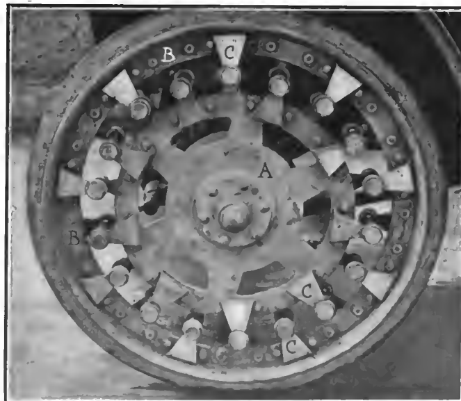
Fig. 2—View of the Schermack spring wheel fitted to car, showing how the flat steel springs are disposed
